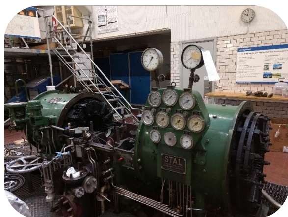
Figure 9: Dismantled turbine, ready for a rebuild to perform another 10 years
