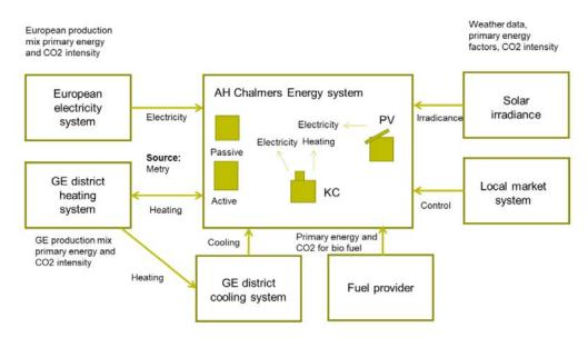
Figure 1: conceptual diagram of the energy flows between the external system and the FED system.
